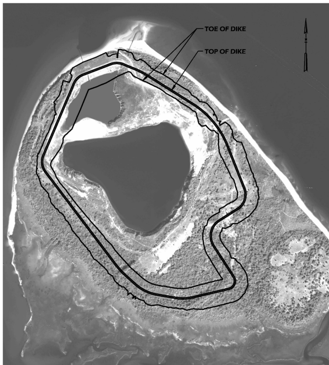
BRANDT ISLAND DIKE RAISE TO ELEVATION 55' NAVD88 ALONG EXPANDED DIKE ALIGNMENT
